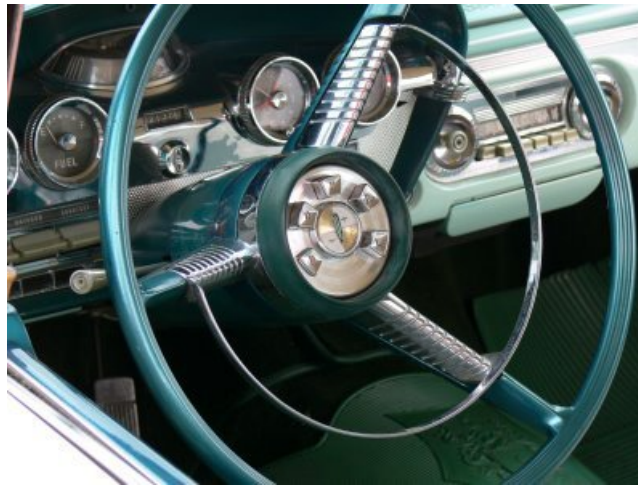
The push-button shifter on the Ford Edsel
